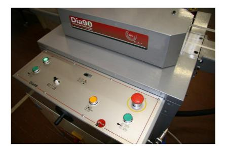
This equipment is designed and manufactured to polish and grind edges in plastic materials such as methacrylate, polycarbonate and similar.
