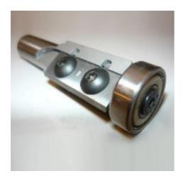
Cutter suitable for removing large amounts of material and for trimming with rough and opaque finishing: working at 18,000 revolutions / minute, cutting diameter with a tolerance of 0.00 mm, coupling diameter 12 mm, height of blades 30mm, replaceable blades sharpened on both sides.
