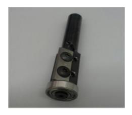
Cutter suitable for removing large amounts of material and for trimming with rough and opaque finishing: working at 18,000 revolutions / minute, cutting diameter with a tolerance of - 0.10 mm, coupling diameter 12 mm, height of blades 30mm, replaceable blades sharpened on both sides. Recommended for work without film, or with thin film. To be combined with Diamond polishing F2.90CD
