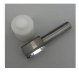
Cutter designed to obtain the preparation of the plate edge to be glued at 89 ° (glues T0 and T1). Works both linear objects such as plates and three-dimensional objects such as already glued boxes
