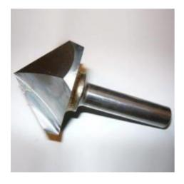
Cutter designed to obtain the preparation of the plate edge to be glued at 44 $^{\circ}$  (glues T2 and T1). It works for preparing the plate edge for cutting at 44 $^{\circ}$
