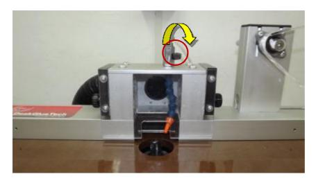
4- The suction and sliding bar settings must always be performed with the machine at standstill
