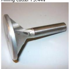
Cutter designed to obtain the preparation of the plate edge to be glued at 44  $^{\circ}$  low thickness or reverse cutting (glues T2 and T1). It works for preparing the plate edge for cutting at 44 $^{\circ}$
