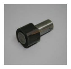
Diamond trimmer height 25 mm: used only to obtain the straight and shiny three-dimensional finishing of PMMA at 18,000 rev / min
