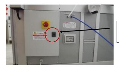
Key to open the panel (allowed only when the machine is not turned on)
