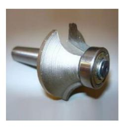
Milling cutter designed for round chamfering at 15° Coupling diameter 12 mm, cutting edge height 20 mm, re-sharpening up to 6 times.
