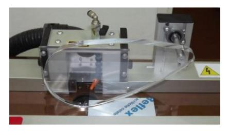
The device allows placing pressure on the material in order to avoid vibration while cutting, but above all it acts as a protection for the fingers and eyes of the operator avoiding the risk that shavings may end up in contact with the operator.
