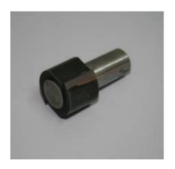
Diamond trimmer height 30 mm: used only to obtain the straight and shiny three-dimensional finishing of PMMA at 18,000 rev / min
