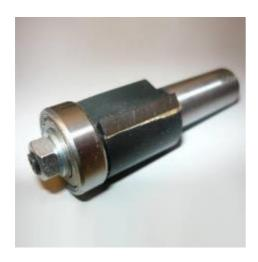
Diamond trimmer, DIA blade height 20 mm, coupling 12 mm: only used to obtain that invisible PMMA glossy finish, it works at 18,000 revolutions / minute on a previously edged piece
