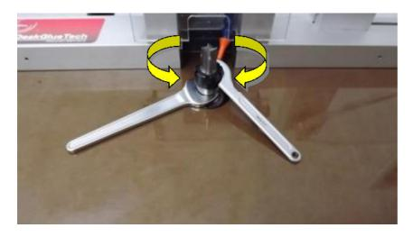
2- unlocking the cutter (be careful to keep the keys firm to prevent damaging or breaking the cutter)
