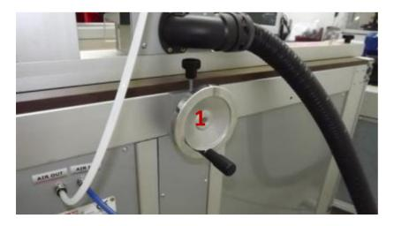
3) Use the 2 keys supplied to loosen it, turning the fastening collar counter clockwise by at least two full turns and then pull out the cutter wearing your protective gloves
